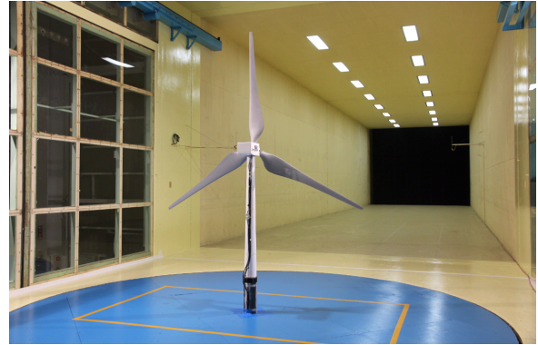
Figure 8: Setup for steady performance testing
