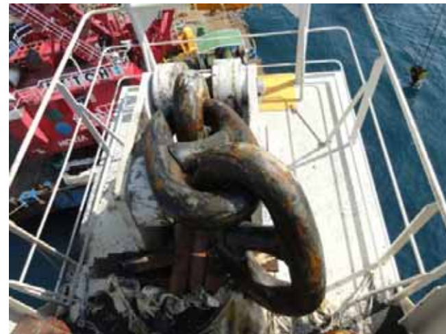
Connecting chain to the floater
