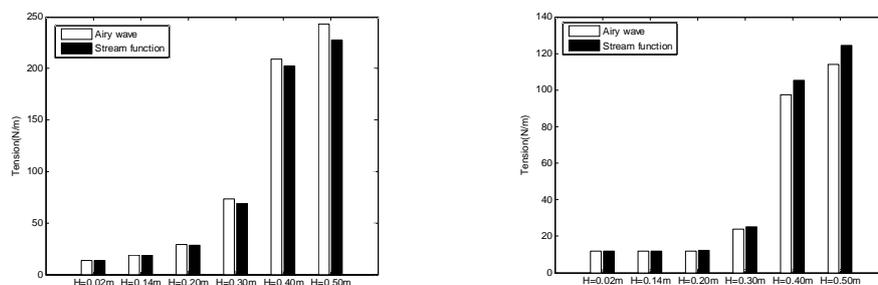
**Figure 5.** Comparison of RAOs of mooring tensions of line 1 (left) and line 3 (right) by airy wave and stream function for different wave heights.
