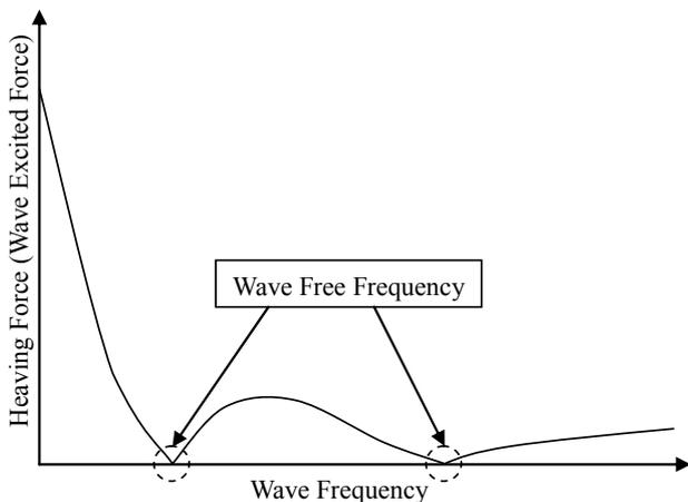
Fig. 8. 2 point wave free frequency
