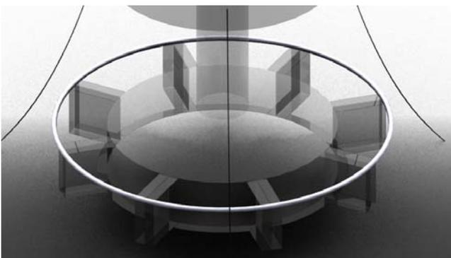
Fig. 6. Detailed image of motion suppression fin
