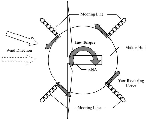
Fig. 5. Balancing of yaw torque and restoring force (Top View)
