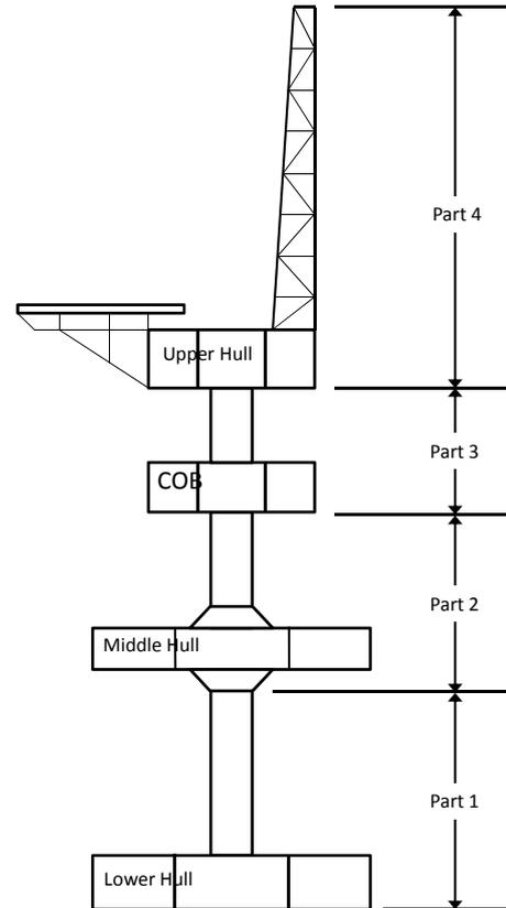
Fig. 13. Block division of offshore substation
