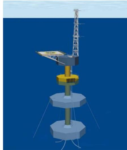
Fig. 9. Isometric view of offshore substation
