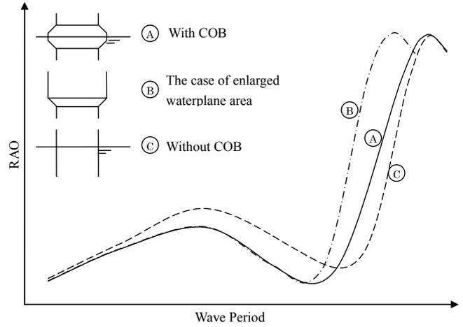
Fig. 4. Schematic curves of heave motion response
