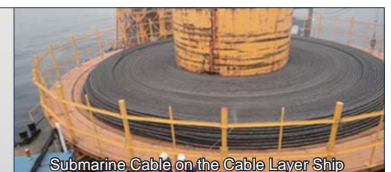
Submarine Cable on the Cable Layer Ship
